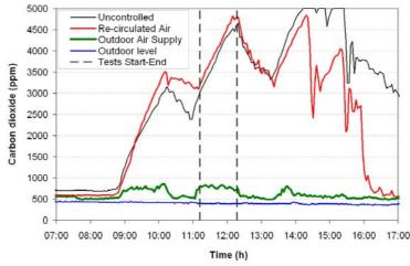
Figure 2. Typical pattern of the  $CO_2$  level inside a classroom at different ventilation conditions on a testing day. The uncontrolled condition reflects  $CO_2$  concentration during a normal school day without any intervention measures.
