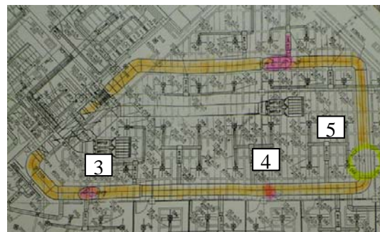
Figure 3. Supply air duct and measurement location
