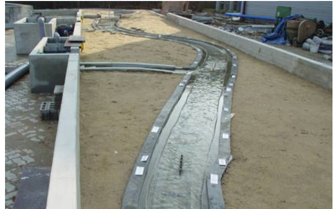
Fig.5. Small scale hydrological experiments were carried out to ensure flow capacity for design flood (longitudinal model scale 1:50)
