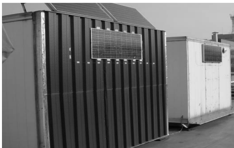
Figure 3. Twin test rooms for PVT hybrid air heating system performance monitoring.
