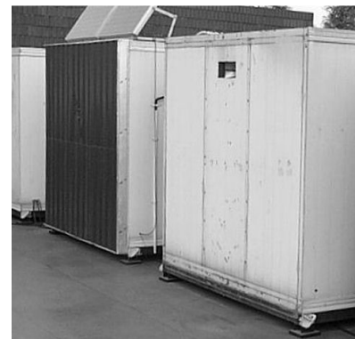
Figure 1. Identical test rooms for monitoring UTC performance
