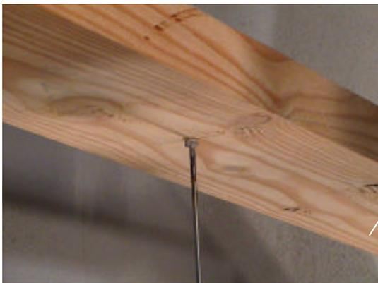
Figure 4: Transducer attached to specimen
