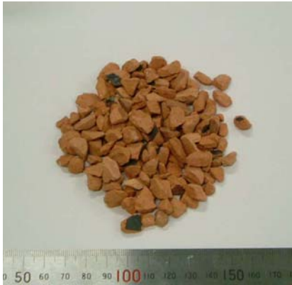
Fig. 1 Particles of Touki ballast with less than 10mm.
