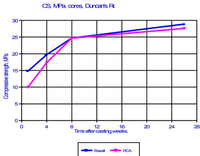
**Figure 5. Core compressive strengths of RC and NC concretes**
