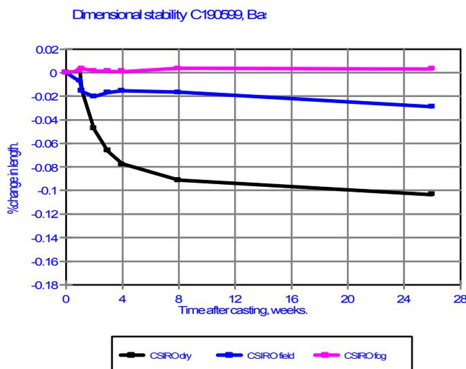
Figure 7. Drying shrinkage of NC concretes
