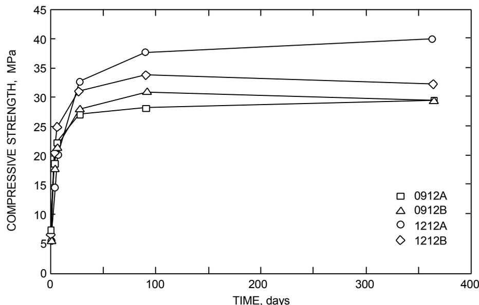
Figure 1. Development of concrete compressive strength with age
