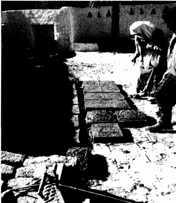
Figure 3: New trial adobes with different mixes: flat and turtle-back
