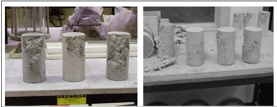
(a). Specimens Without Fibre
