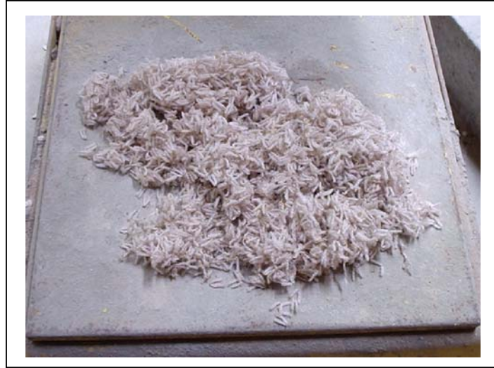
Fig.2: Nylon Yarns Disassembled from the Face Layer of the Wasted Carpet
