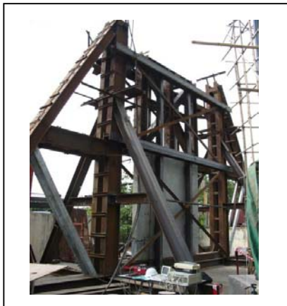
Fig.8 Cyclic load test for precast wall panel
