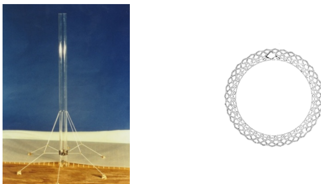
Fig. 4 Model of a 600 meter high solar chimney and its cross sectional plan representing a porous organic form (source: the M. Elnimeiri)
