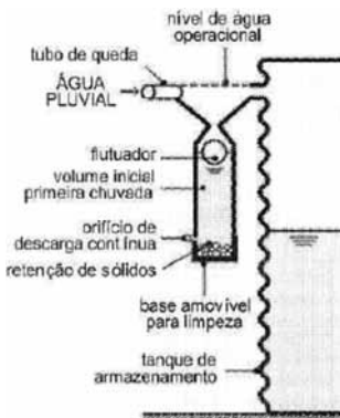
Fig.10: Schematic of a diverter first rains [7]
