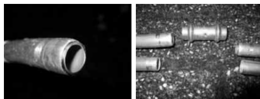
Fig.7: pipe end(s) with burr
