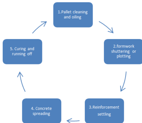
Fig.2. Producing loop of precast concrete
