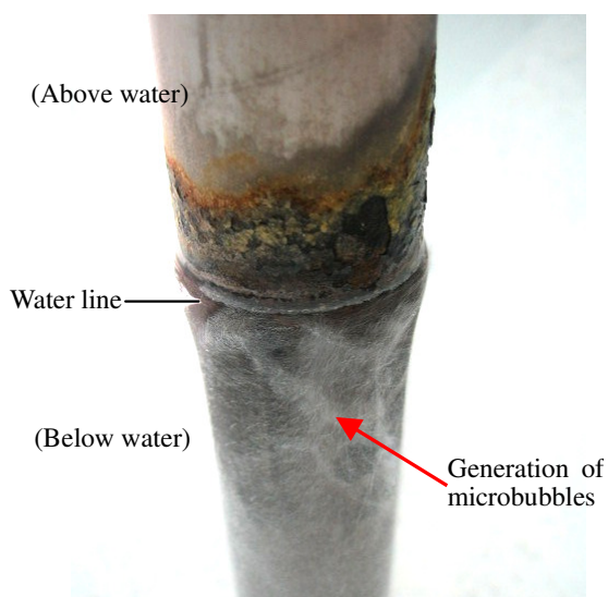
Figure 3 - State of active dissolution of handrail in bathtub No. 3, About 12 months use
