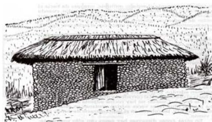
Figure 9 Lenca's house of rock and manaca's roof
