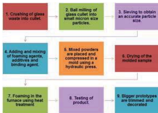
Figure 1. The flow diagram of the production process of foam glass prototype
