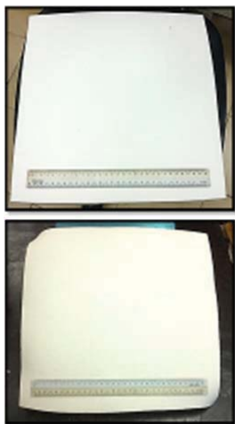
Figure 11. Big foam glass prototypes produced at 800-825 °C
