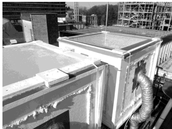
Figure 2. The ETFE cushion (left) alongside the double glazed unit (right)
