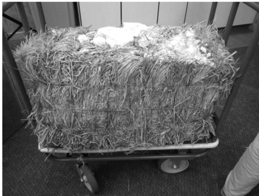
Figure 2. Bale recently removed from Nebraska dwelling built in 1913
