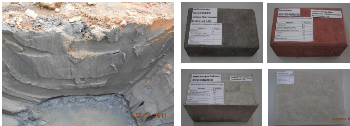
Figure 10: Marine Mud Stabilization for Back-filling and building materials including paver blocks, planter curbs and roof tiles
