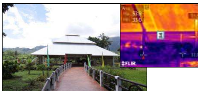
Figure 9 Before: The heat of the sun hits the tent (conference pavilion) roof and the surface temperature of 55 °C
