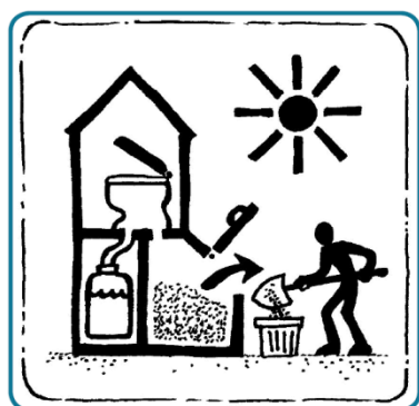
Figure 5 Elevated temperature from exposure to the sun promotes dehydration and pathogen die-off
