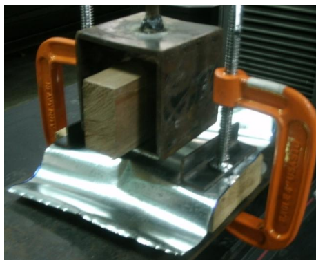
Figure 5 Combination of roofing, fastener, purlin test set-up
