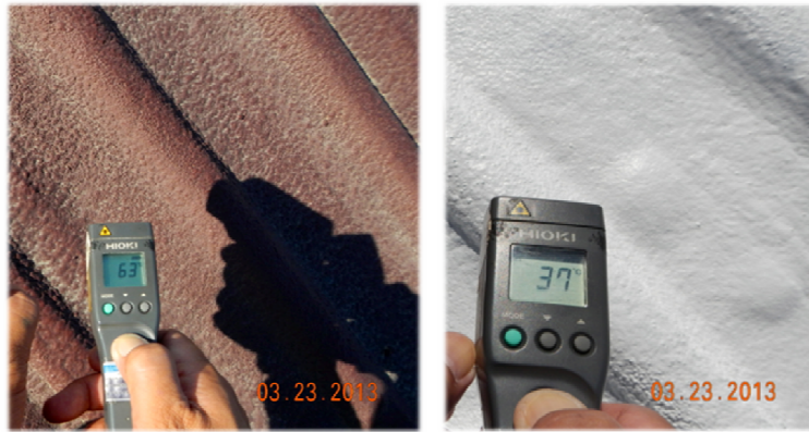
Figure 4 (before) Dark brown colored roof (after) White Elastomeric Paint coating on top of the existing brown colored
