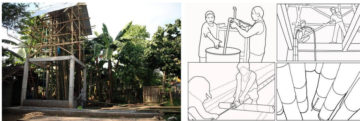
Figure 7 Vertical Soak Diffusion (VSD) plant adjacent to the bridge's site (left) and illustrations of the treatment process (right)
