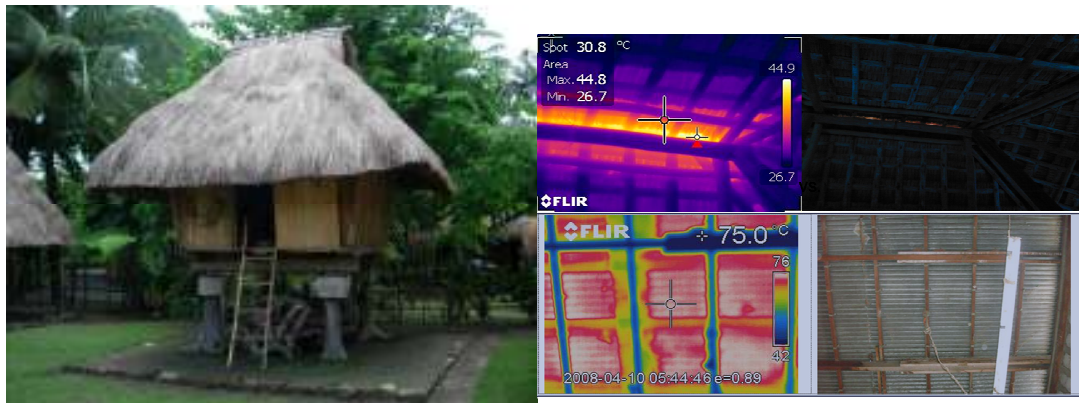
Figure 2 (left) An “Ifugao house” (right) Heat gain comparison between cogon roof and galvanized iron roof
