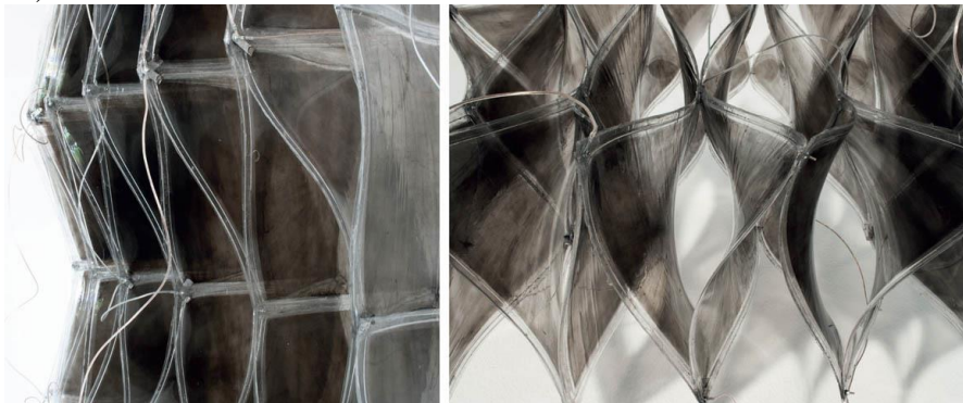
Figure 2: ‘Shape Shift’ prototype, consisting of 36 individual EAP elements, as exhibited at the Gallery Stark Art in Zurich, (Source: Addington and Schodek, 2010)
