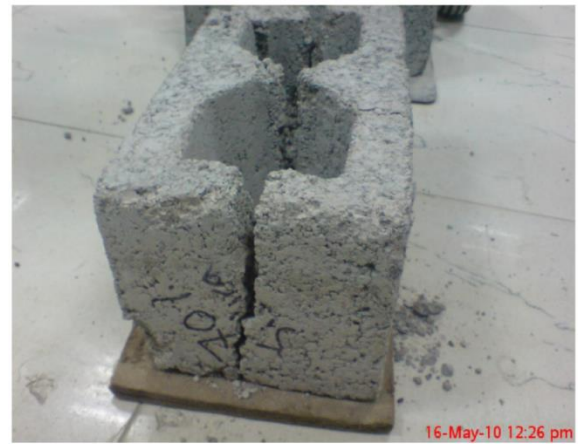
(b) failure mode of blocks
