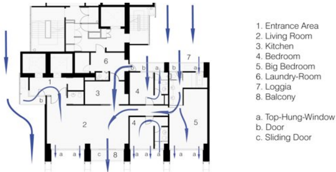
Fig. 13. 29th Unit C Floor Plan the MET with Openings Categorization © Ferdinand Oswald, WOHA (9)
