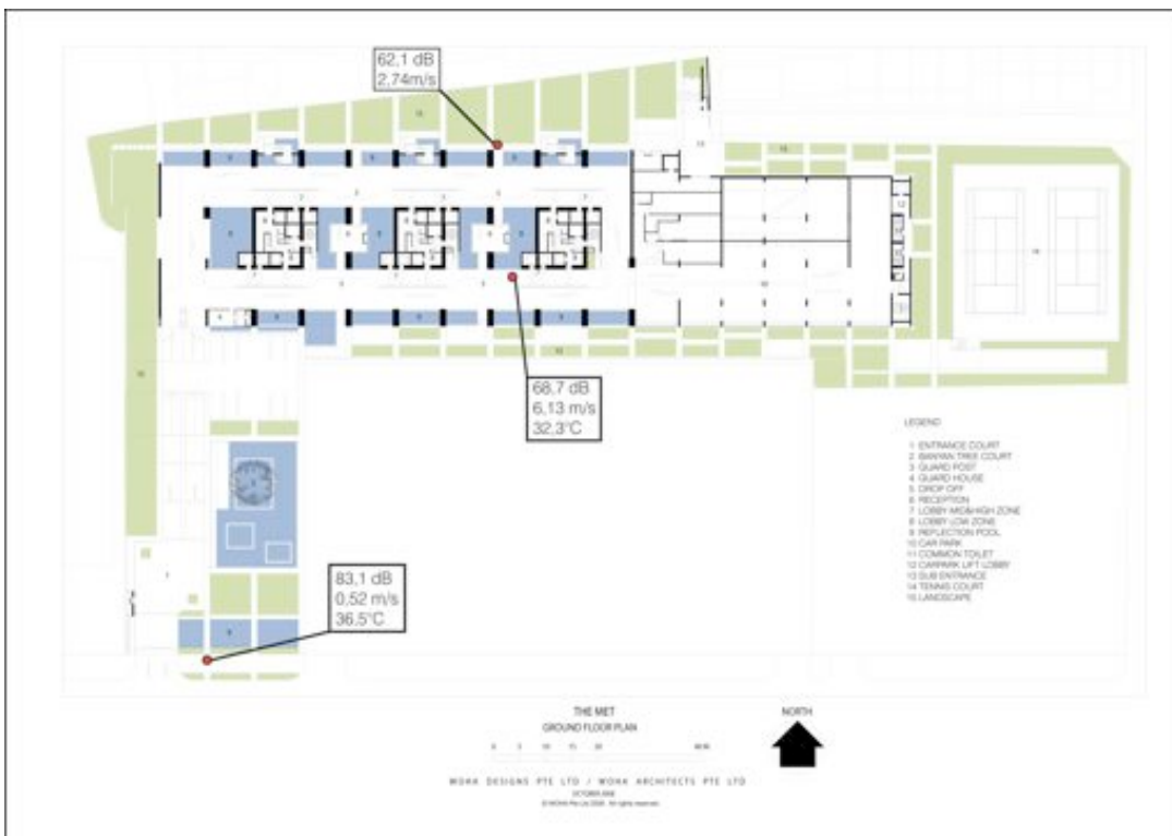
Fig.11. Ground floor the MET - Wind Speed, Decibel and Temperature © Ferdinand Oswald, WOHA (7)
