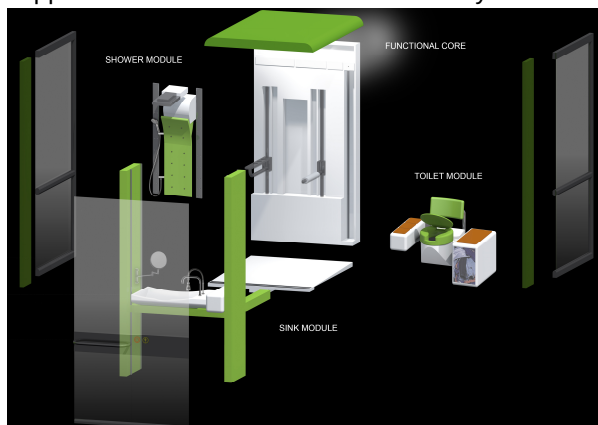
Fig. 10 The exploded BCUBE: the functional core, the wc, shower and sink components, the enclosure
