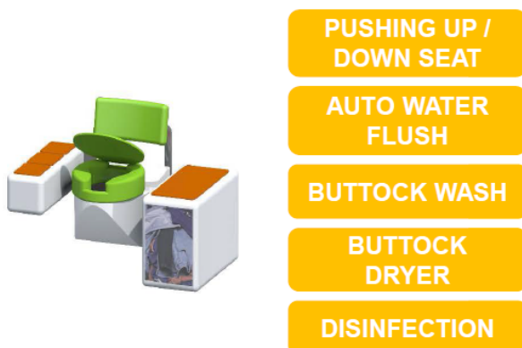
Fig. 3 The WC component, along with its possible functionalities
