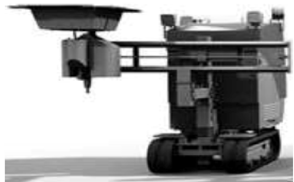
Fig.3. Mobile robot for hydrodynamic concrete and metal treatment
