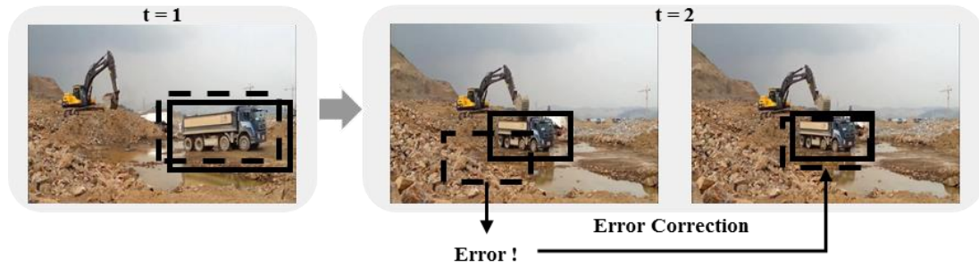
Figure 3: Error Correction Based on the Functional Integration a Detector and a Tracker.
