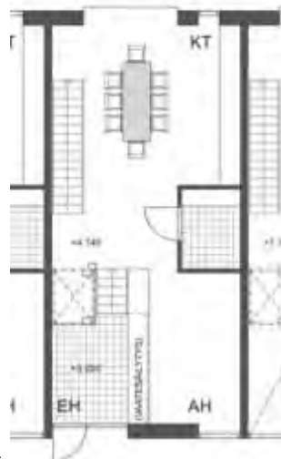
Fig. 6. The main floor is planned half a storey height above the street level. The difference of level is managed inside the apartment. A space for a possible lift is in the plan. (Jätkäsaari, A-konsultit)
