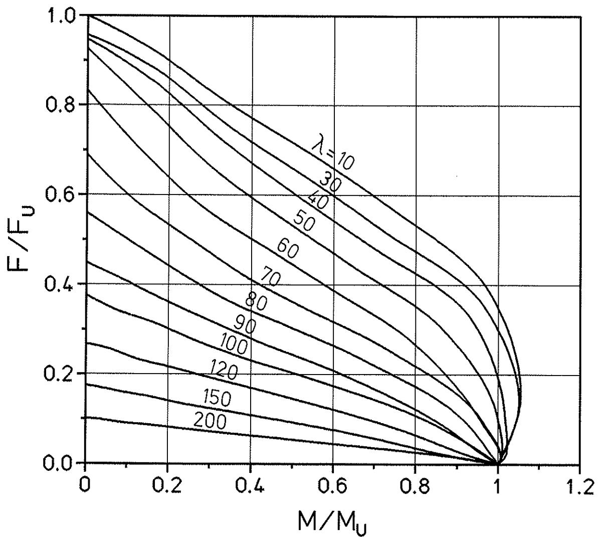
Fig. 6 Moment - normal force - interaction for glulam columns grade II
