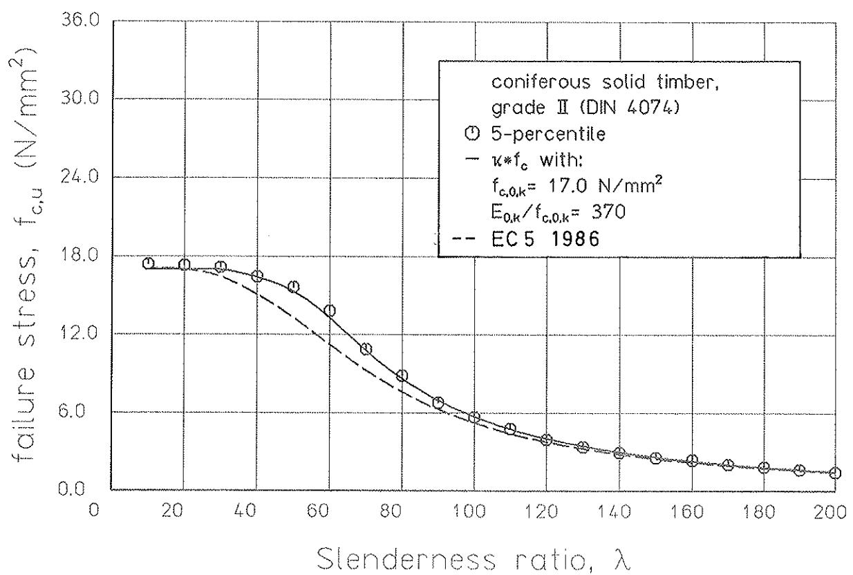
Fig. 5 Characteristic buckling strengths (failure stresses) for solid timber columns
