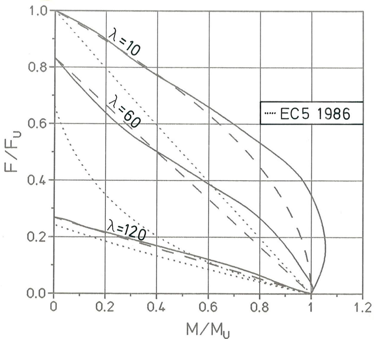
Fig. 7 Approximations for eccentrically loaded columns
