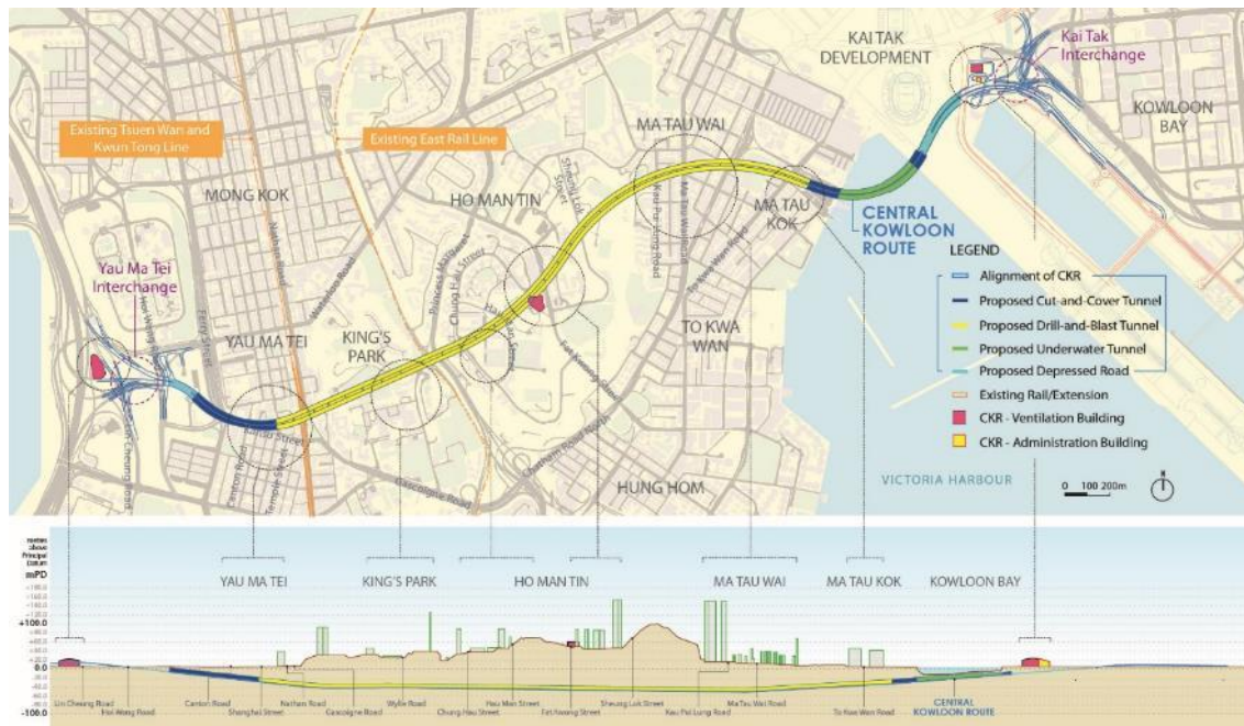
Figure 1: Layout plan and longitudinal section of CKR
