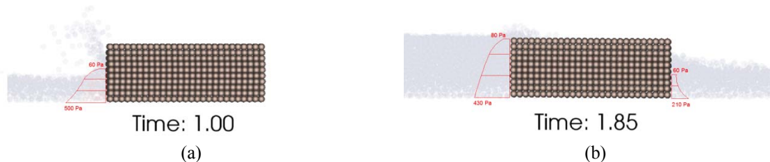
Figure 7 Computed pressure profile on the upstream and downstream faces of the solid at t=1.00 s (a) and t=1.85 s (b). Case TS07801, diameter 78 mm and slope 1%
