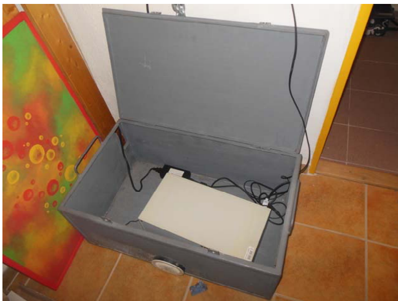
Figure 3 Data logger AHLBORN ALMEMO A 5690-2 TS placed in lockable steel box
