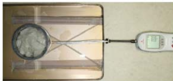
Photo 1 Measuring the horizontal force with a push pull gauge
