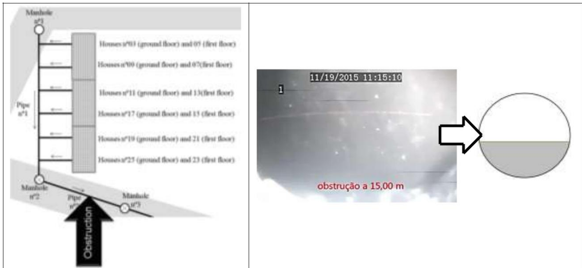
Figure 16 Detail of obstruction observed on the second real time video
