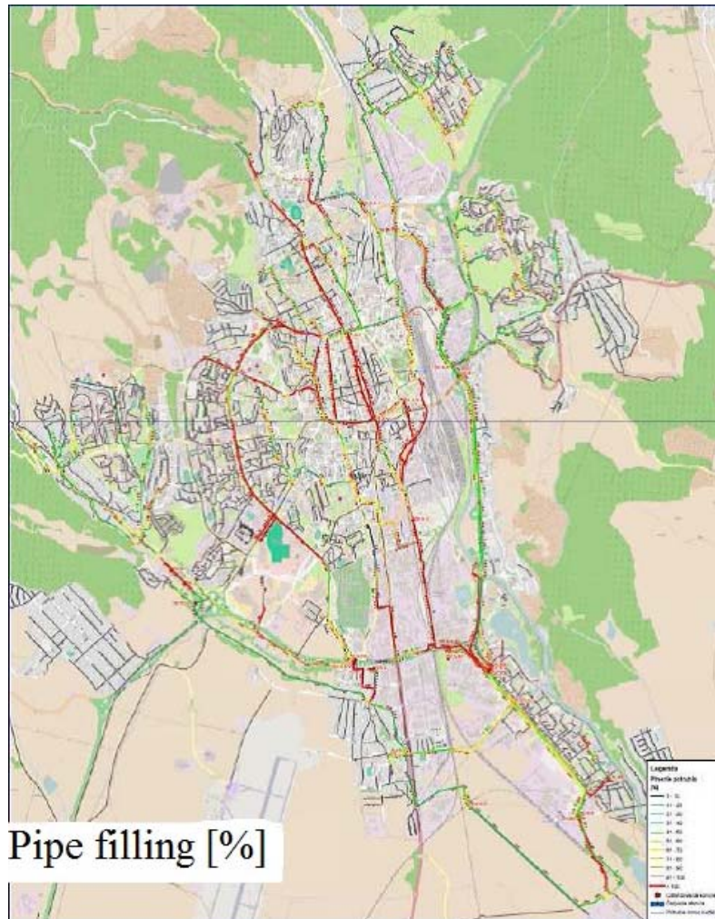
Figure 9 Pipe filling in % during measurements
