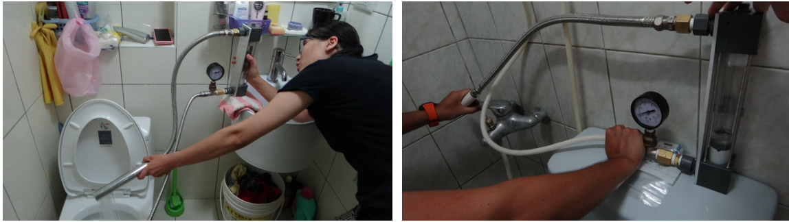
Fig. 5 The field Survey was operated with measure device in different households
