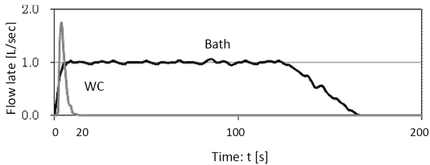
Figure 1 Discharge characteristics of fixtures
