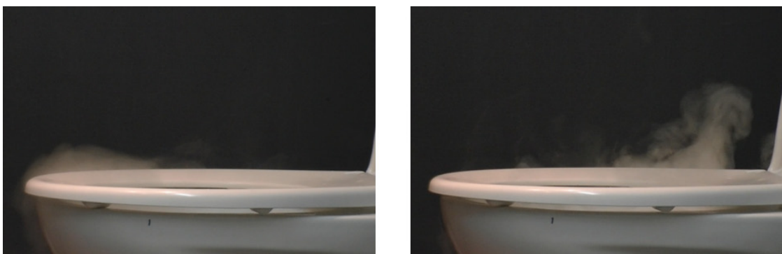
Figure 5 and 6 -Flow visualization with cold water: start and end of flushing
