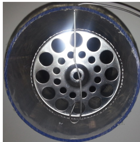
Figure 3: Non-intrusive bioaerosol sampler
