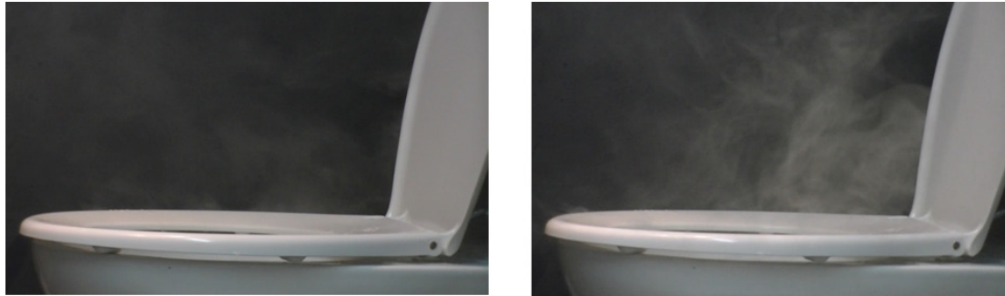
Figure 7 and 8 - Flow visualization at 26 °C: start and end of flushing
