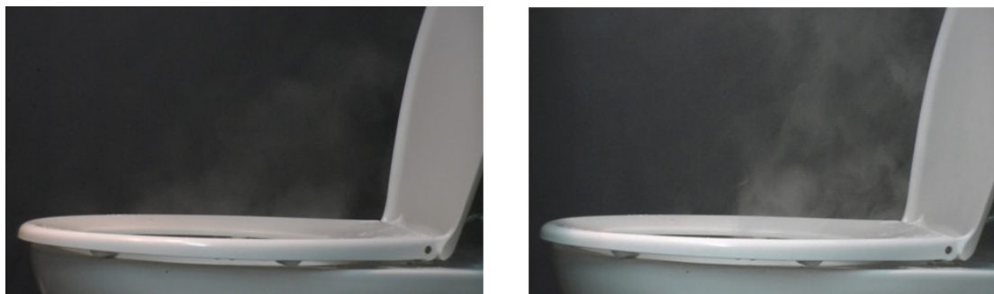
Figure 9 and 10 - Flow visualization at 32 °C: start and end of flushing
