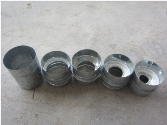
Fig . 8 Variable diameter short pipes on the top of vertical pipe
