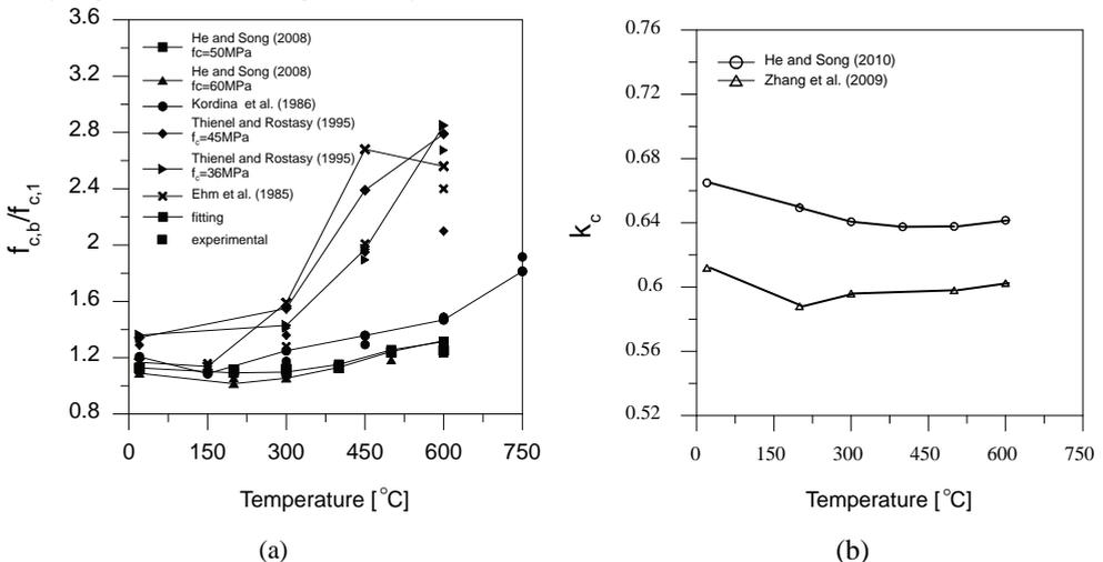
Fig. 2. Results of the fitting procedure: comparison of (a) uniaxial-to-biaxial strength ratio and (b)  $K_c$ .
