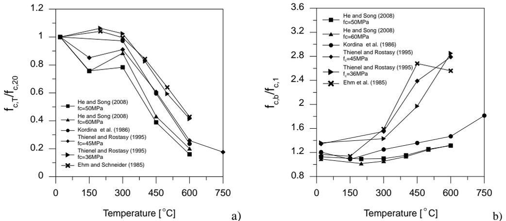
Fig. 1. Test results considered in the fitting procedure: a) normalized decay of the uniaxial compressive strength; and b) ratio between biaxial and uniaxial compressive strength as a function of temperature
