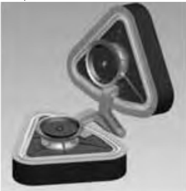
Fig.7. Two robot modules connecting by a hinge in +90°
