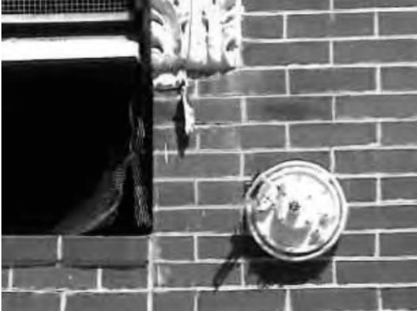
Fig.6. City-Climber prototype-I approaching a window on brick wall
