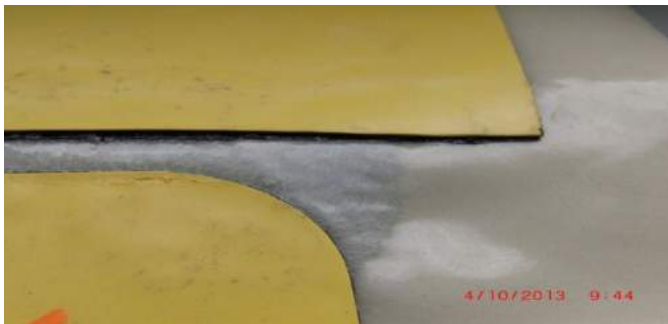
Figure 12: Two types of new membranes heat welded to a sample from the Reussport tunnel.
