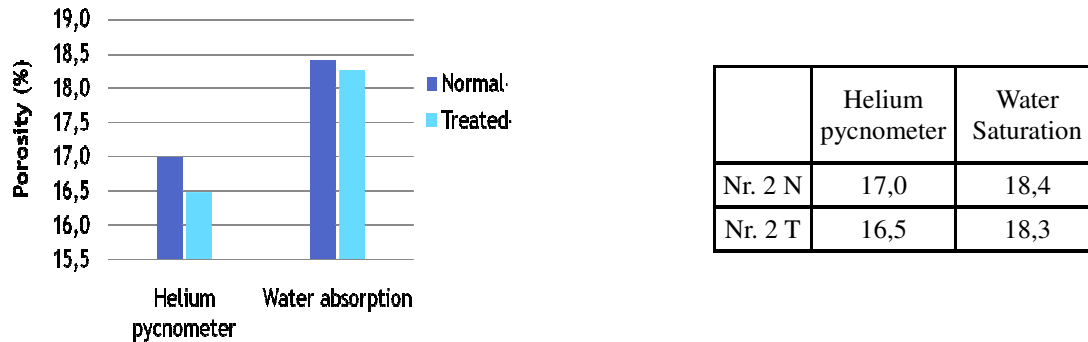
Figure 8: Porosity diagram and table of Mix Nr. 2 for normal (N) and treated (T) aggregates
