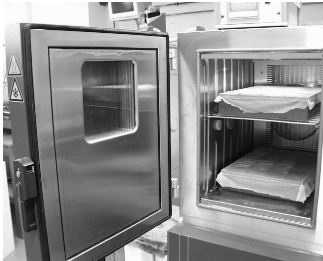
fig. 1: climatic chamber with sample arrays for the tests at different temperatures and air-humidities.
