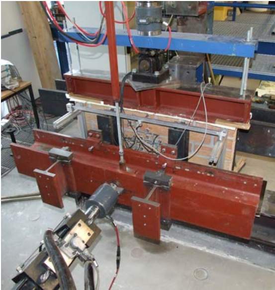
Figure 5: Test setup to determine the flexural tensile strength parallel to the bed joints under superimposed load (left) and load deflection curves (average centre deflection) of the masonry walls made of solid bricks W2 with normal mortar at different superimposed load levels
