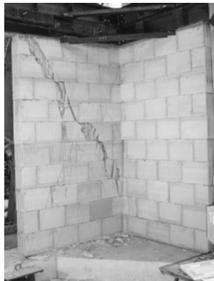
Specimen V0a after the final test
