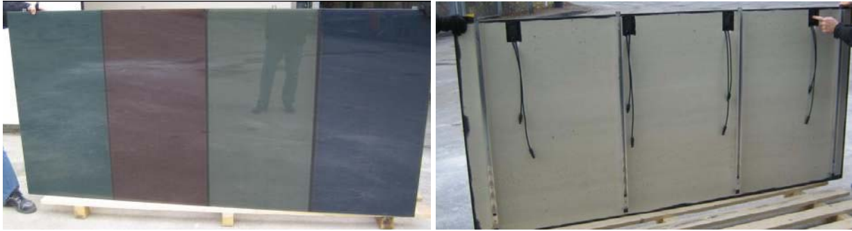
Figure 4 Aged PV-element; left: Front with optical opacities of the composite film at the upper edge; right: Back-side with junction boxes and aluminium substructure
