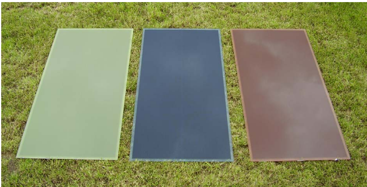
Figure 2 Prototypes of coloured thin-film PV modules produced for façade cladding elements using inorganic coated cover-glasses.
