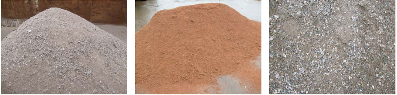
fig. 4 to 6: Crushed recycling material, fraction 0/5 mm calcium silicate material, brick material and concrete material Brockmann Recycling GmbH, Nützen, picture: TerraTextura GmbH, Soest
