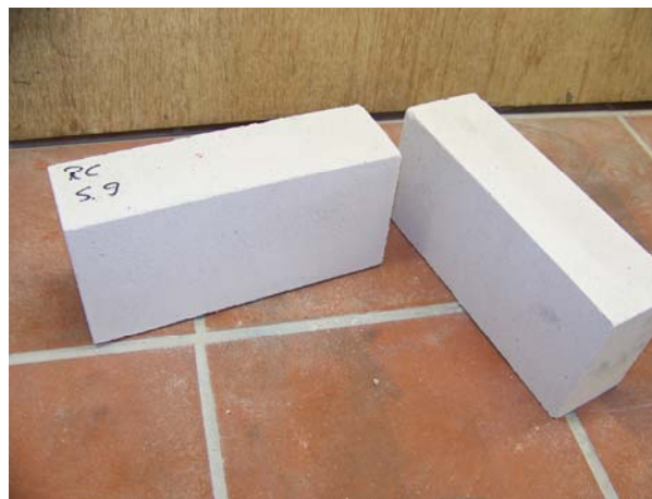
fig. 11: Specimen of the series 9 with 50 wt.-% of calcium silicate of the fraction 0/2 mm (example)
