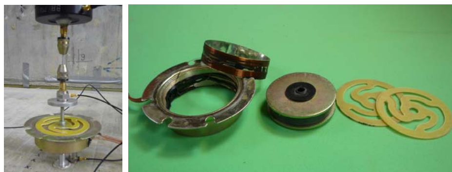
Figure 2: Model setup without passive elastic interlayer (left) and elements of the electro-dynamic actuator (right).
