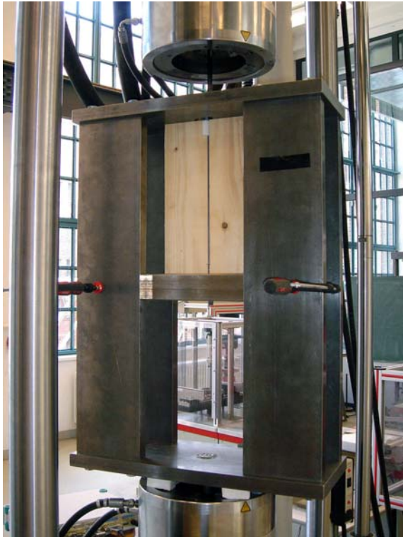
Figure 2: Pull-out test on a wood/CFRP-composite test specimen
