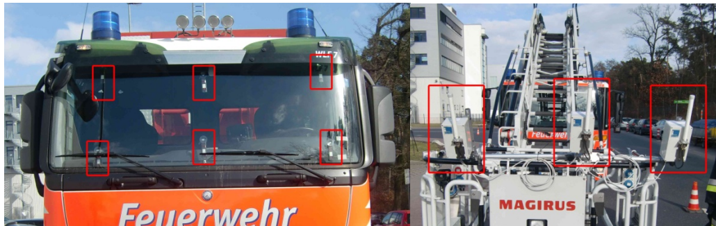
Figure 6: Test equipment for range / accuracy measurement (left: Truck stocked with RFID-tags; rights: Turntable ladder stocked with i-SATs) (Image source: Hr. Fabian, Identec Solutions)
