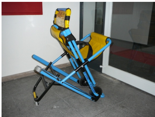
Figure 2: Evacuation chair – a complementary or compensatory means of transporting physically disabled persons up or down emergency staircases [Photo: Grossmann]
