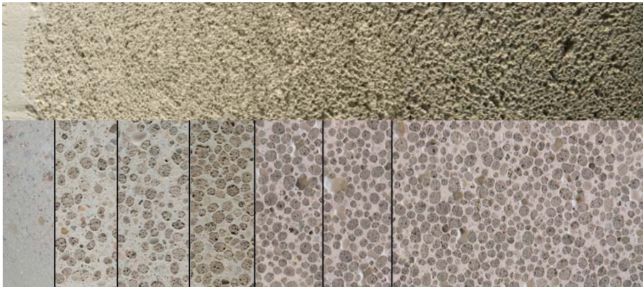
(Figure 2 top: density graded aerated concrete, source: ILEK; Figure 2 bottom: homogenous concrete mix with graded density for material testing [2], source: ILEK)
