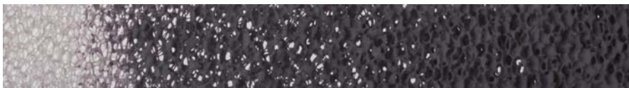
(Figure 5: Graded infiltration of reticulated polyurethane foam with cement slurry for the varying of stiffness, source: ILEK)
