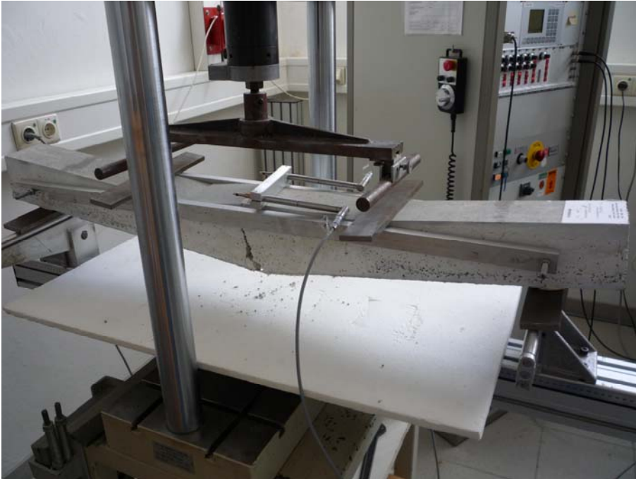
(Figure 3: Functionally graded slab specimen, source: ILEK)
