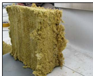
Sample with considerably reduced resistance to pressure
