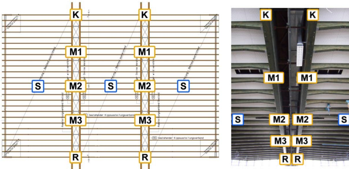
Figure 6: School gym Murnau, monitoring system: Schematic diagram of the locations of the snow cushions (S) and the deformation measurement system consisting of the camera units (K), measuring points (M1-M3) and reference points (R)
