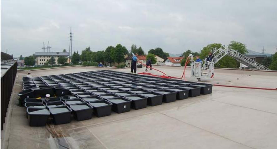
*Figure 10: Artificial load on the roof of the school gym in Murnau, consisting of 154 buckets of the size of 90l, filled with water*
