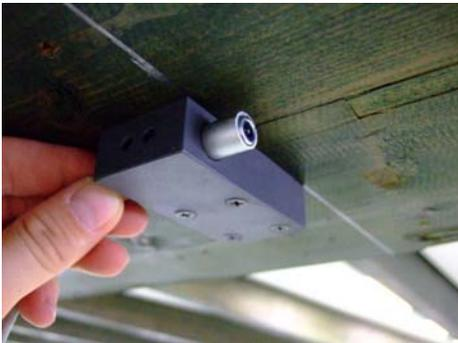
Figure 8: LED of a measurement point during installation with steel casing.
