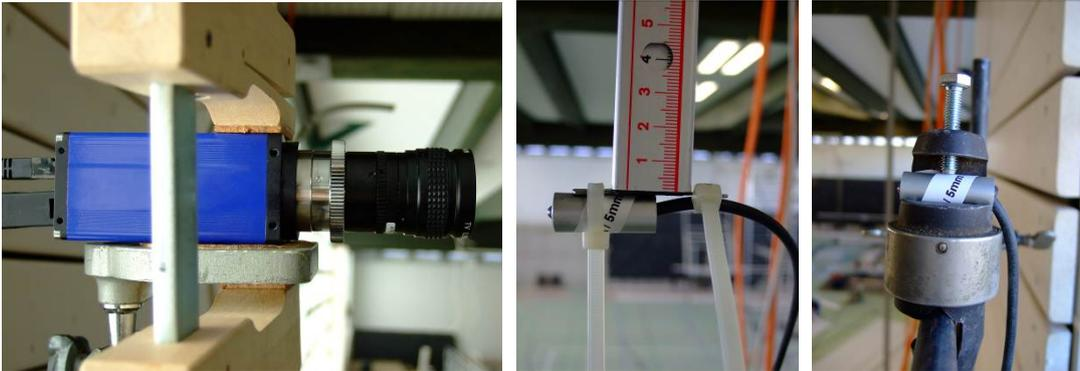
Figure 2: Preliminary test: Camera (left), movable measuring LED (center) and reference LED (right)
