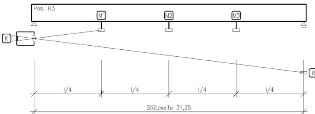
Figure 5: School gym in Murnau, deformation measurement system: Arrangement of camera (K), measurement points (M1-M3) and reference point (R)
