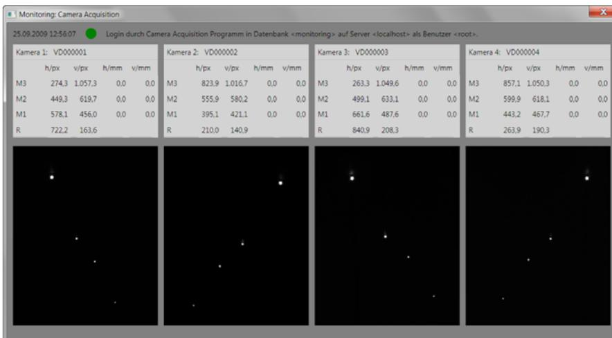
Figure 9: User interface of the measurement software Camera Acquisition with images of the LEDs mounted on the four main beams (bottom), deformation values (center) and warning notification area (top)
