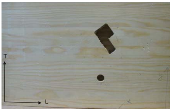
Fig. 1 Large pine wood specimens (specimen X1124) with L-shaped defect (back side)
