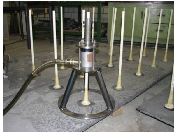
Figure 5: Adhesive tensile strength test of FRP-concrete bondage
