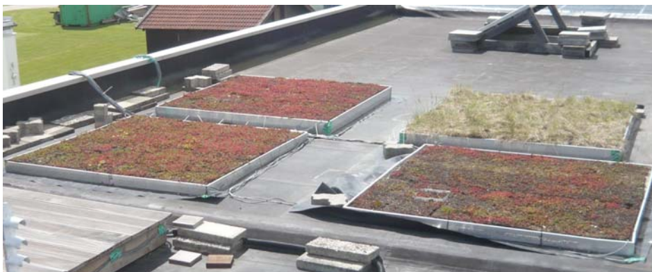
New field tests in Holzkirchen with different substrate types and thicknesses.
