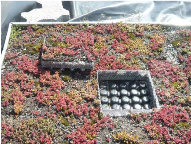
Basket for manual weighing and registration of the substrate moisture content.
