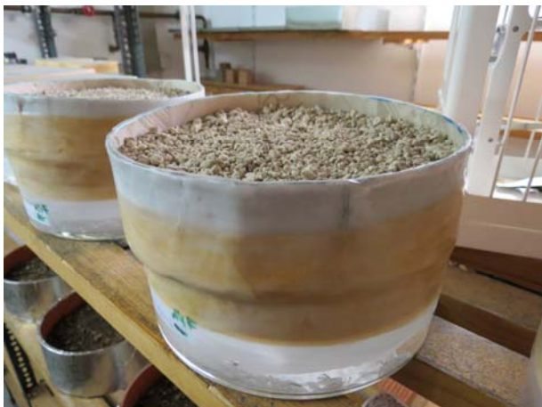
Determination of the material properties of the different substrates in the laboratory (here: diffusion resistance)
