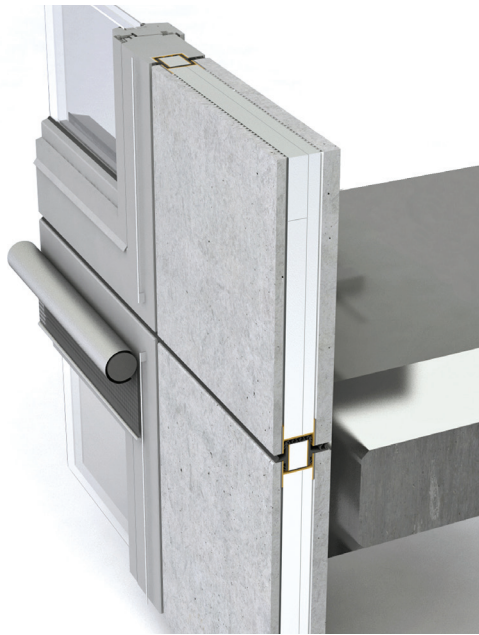
Fig. 11 Axonometric drawing of a facade detail, s.: HTWK Leipzig
