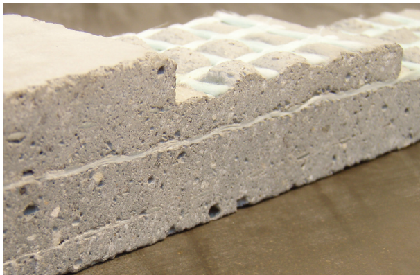
Fig. 3 Material sample textile reinforced concrete, s.: TU Dresden
